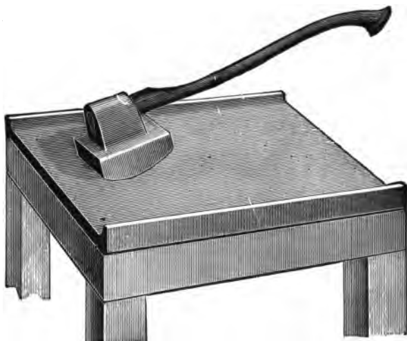
FIG. 35.—BUCK BOARD AND MULLER.
